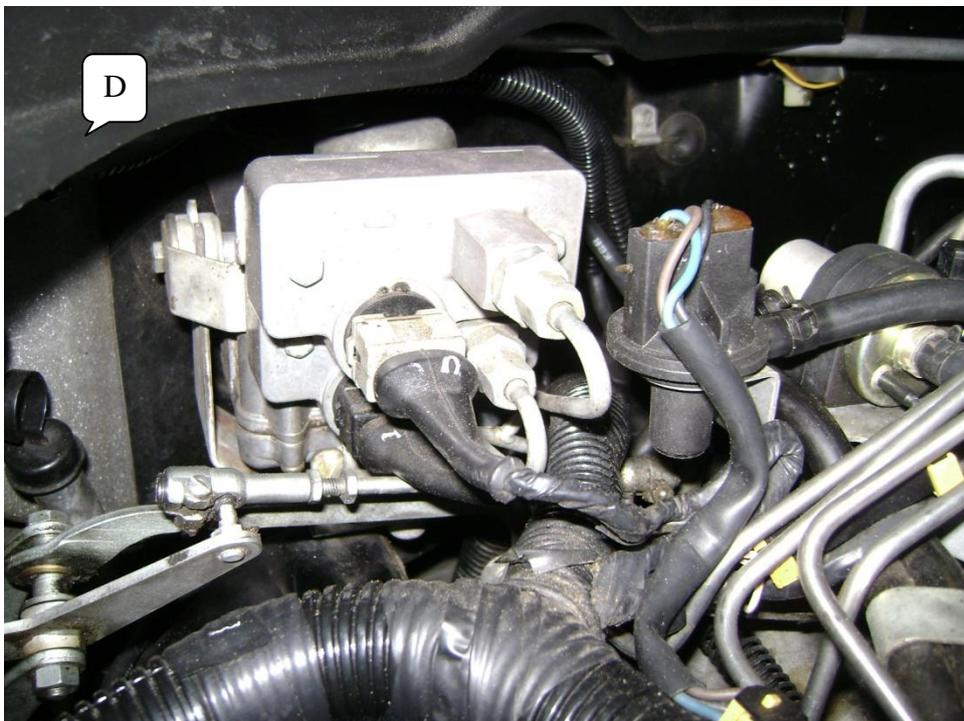
This is the air pressure transducer see 'D' in the pic. Transducer as a word has been around for a long time but little used apparently. It simply means a device for converting one type of energy into another.
