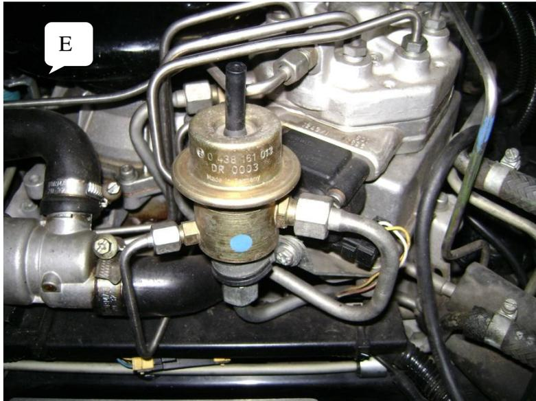
The central bit 'E' here is the fuel pressure regulator. If you are not familiar with fuel injection it comes as a shock to find that the system runs at pressures in excess of 85 psi! This compares alarmingly with the old SU pumps and the Pierburgs running at a pound and a bit! The fuel system is of course recirculating and this little gadget makes sure that the main working bit, the Fuel distributor seen behind the regulator has a constant correct pressure.
