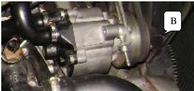
The Air Pump. 'B' This is a gadget spawned by those people who object to being choked by automotive emissions. They have been on the Shadows for years particularly for those cars delivered to the West Coast of America. Given the speed that the engine has to suck in a mixture of fuel and air, set fire to it and get rid of
