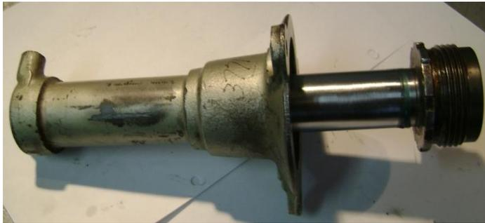
The second picture shows the ram fully extended some three inches. The bottom of the plunger is threaded to screw into the top of the spring holder. The turning is effected with the aid of a 'C' spanner. Very early cars regrettably used a fine thread on the plunger head which with the aid of a little rust requires the patience of Job and the strength of Hercules to unscrew it. When replacing the assembly think of the next operator and liberally coat the thread with anti-seize grease.
