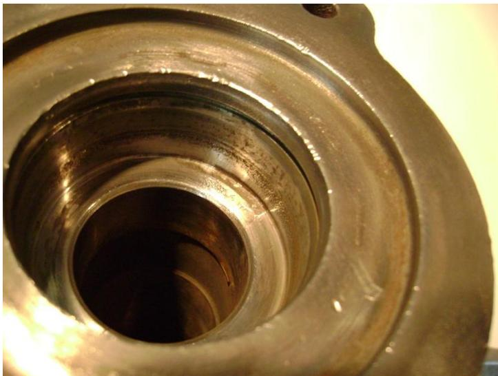
At left can be seen the recess for the seal in the ram housing. The upper groove carries the retaining circlip. With the Chapman seal it is important that the walls of this recess are smooth to aid sealing with the seal's outer 'O' ring.
