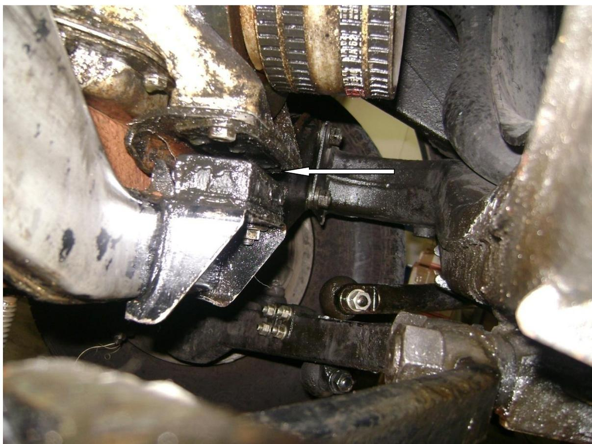
The front end of our cars' engines are notoriously incontinent. This is due to a quaint sealing arrangement between the two castings that close off the front of the engine. The sealing material used hardens and shrinks and oil escapes – all over the front mount. If circumstances prevent correction of this leak and the mount is replaced, wrap it in stout plastic for protection. In the above example the engine has been cleaned albeit too late – the damage has been done.
