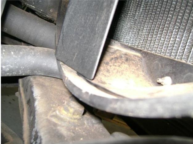
Here note the almost nil clearance between the fan and cowling at the bottom. The location of the engine in post-55 vehicles has always intrigued me. The rear mounts of the vee eight are adjustable (at least vertically) and the front mount sometimes has and sometimes hasn't an extra spacer or two to lift the front of the engine. But I have yet to see any guide as to where the engine should actually sit!
