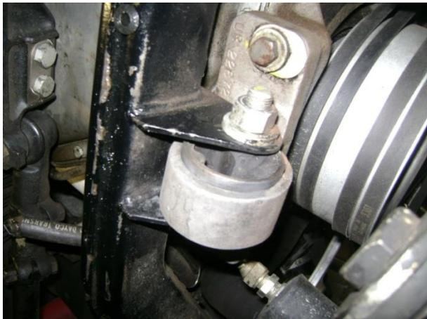
And here is the culprit, the front engine mounting. These circular mounts were used for a while but presumably proved unsuccessful. Note the mount insert is protruding here about 1/4". In addition the whole insert has rotated lowering the engine about an inch.
