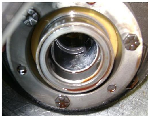
Above. The torque converter normally bolted to the 'flywheel' is a sealed unit (by welding). If you get nasties in the sump and either overhaul the box yourself or have it done, be sure to have the unit opened, flushed and repaired since it is impossible to get muck out of it. It follows that you should also ensure that the transmission oil cooler is flushed.
