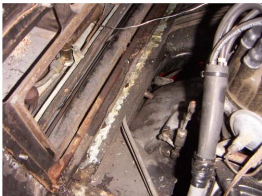
Another source of water is the condensate from the air conditioner evaporator. When the ice that forms on the fins melts it should run out the small pipe seen in the middle of the picture at left. This is the source of that embarrassing trickle that everyone puts up with when the car is parked on a hot day! If this tube blocks the water banks up and once more you have a flooding problem.
