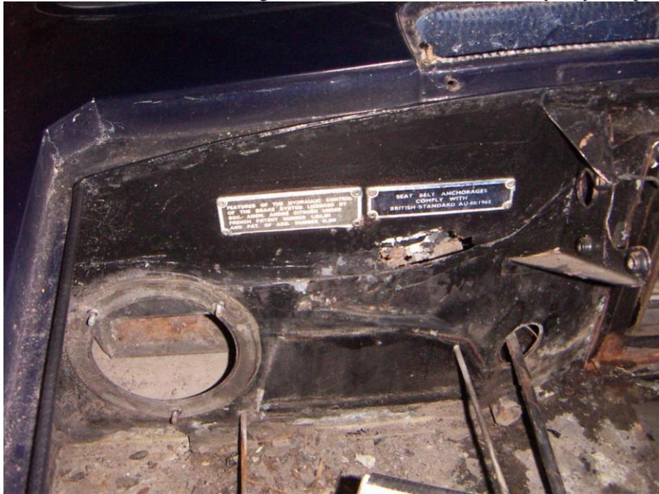
All the pretty bits stripped away and we start to see the damage caused by blocked drains. I suspect this was an English delivery which means the poor thing had to cope with salt water as well. The drain pipe can be seen under the speedo cable which is the rod like thing going through the large hole at the right.
