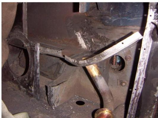
Unfortunately owners frequently cannot be bothered to keep the foam filter under the air intake grille intact, twigs bugs leaves etc get in and the drains block.
