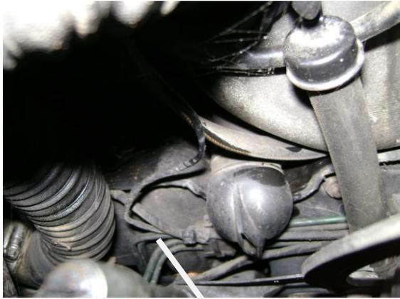
The plenum actually extends to almost the outside limits of the engine compartment with only a small divider provided to stop the water sloshing right across in the event of a drain blockage. If the water does get across this, the first you know of it is usually water on the feet from the re-circulating outlets. You can see these if you get down on your belly and look up under the dash. They are at either end of the ducting.
