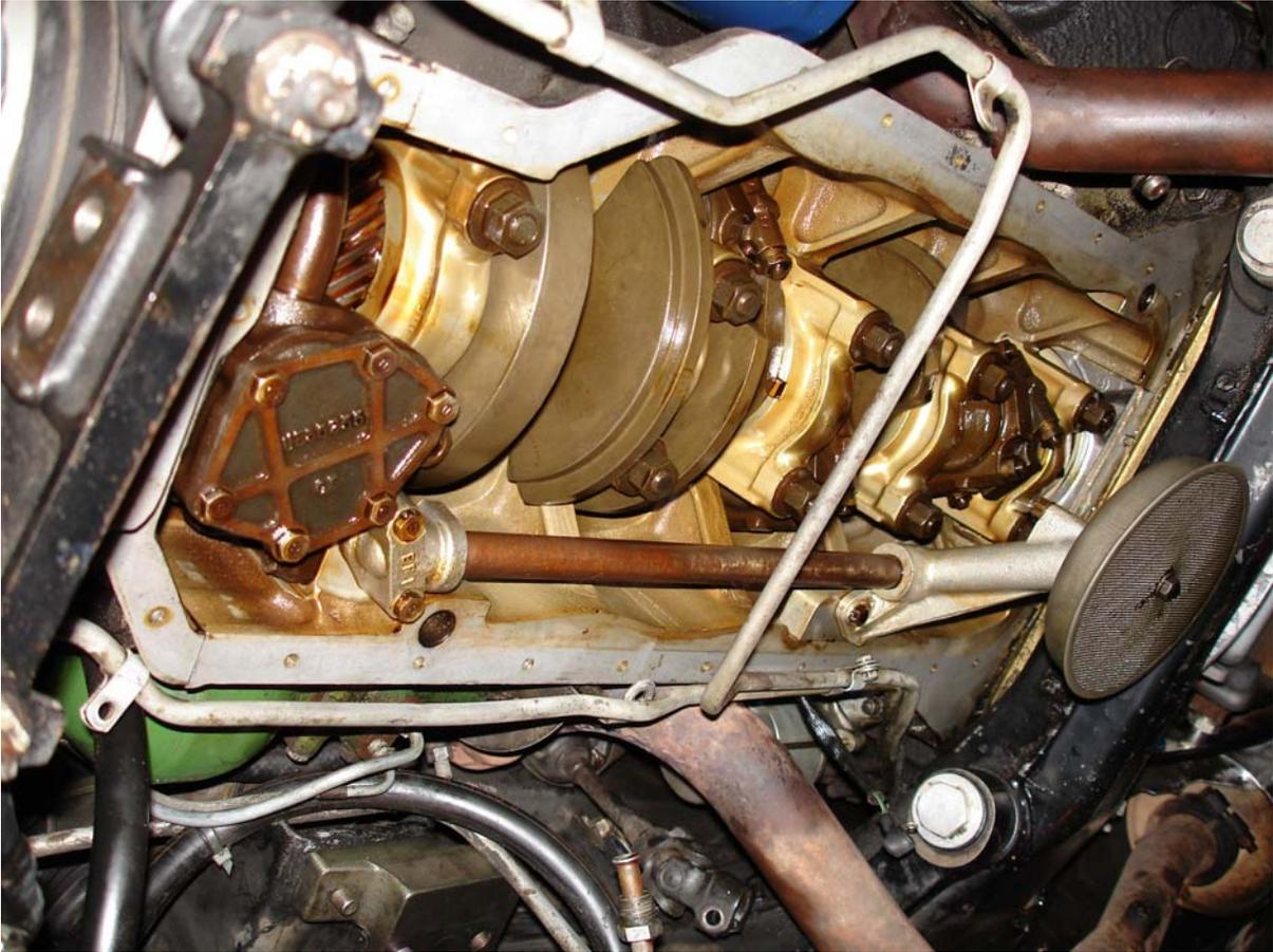
engine can be lifted an inch or so clear of its mounts to get at the 'side' bolts over the cross member.
