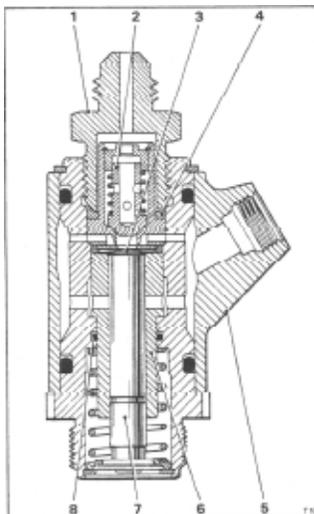
And here is the pump in section. The dark dots are the errant 'O' rings. There really is little to go wrong with these pumps other than they get clogged up through neglect.
