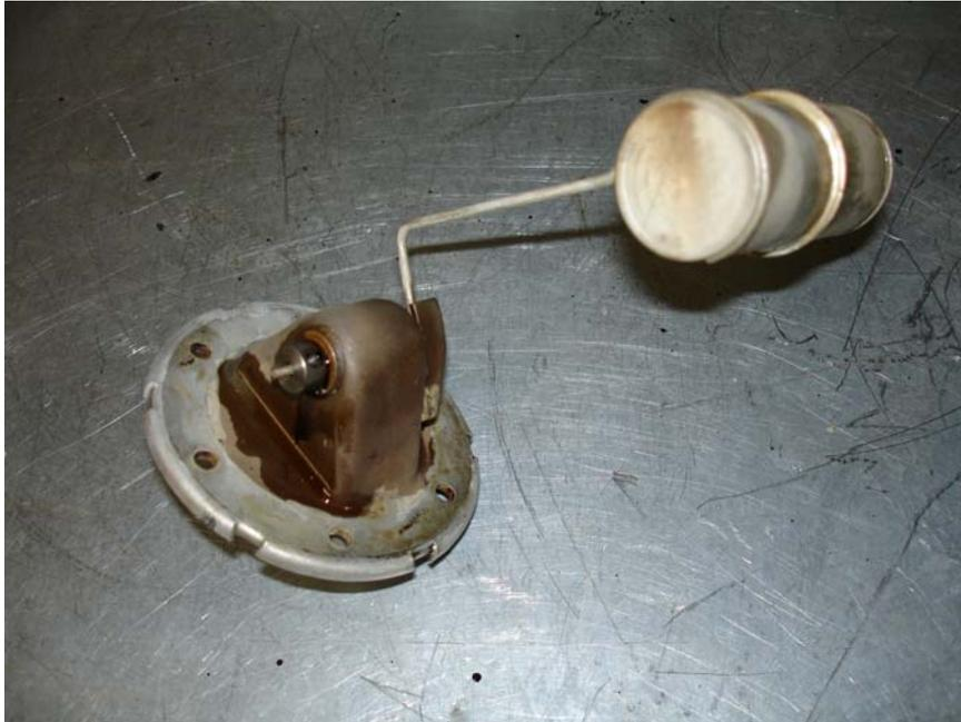
This is the float that bobs around in the sump to tell you what is the oil level. There is a new thin plastic sheet gasket supplied for the joint between the float assembly and the side of the sump which at last appears to have stopped the perpetual leak that has existed on all preceding cars. When you remove the retaining screws note that each one has a star washer and a very thick washer under the head. The thick
