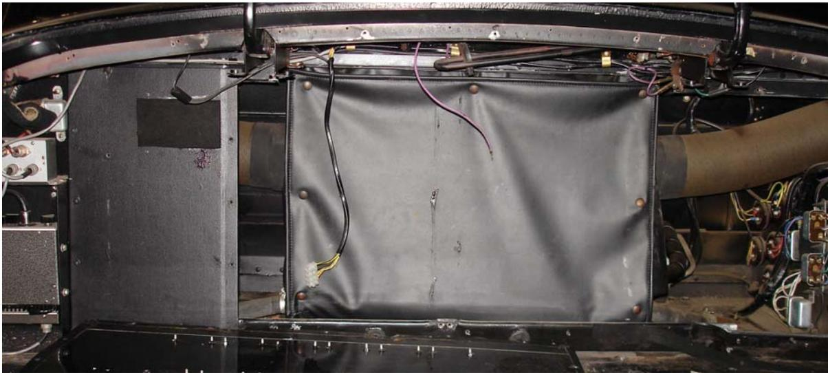
And here is the rear boot air conditioning unit. The delivery pipes seen directed to either side of the boot connect with plenums delivering cooled air to ceiling ducts and controlled ducts at either side of the rear parcel shelf.
