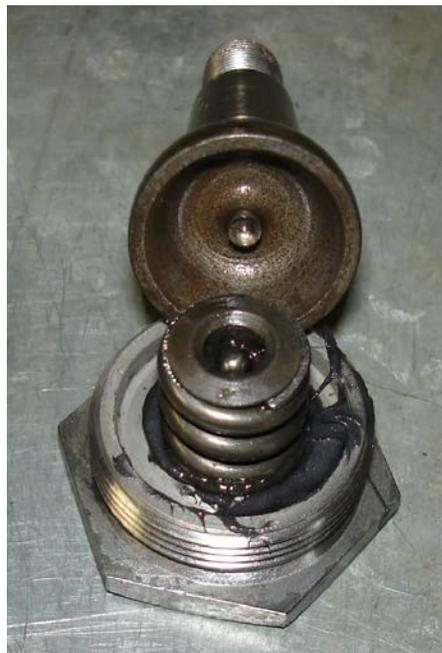
removing the retaining nut, had it been left unscrewed there would have been a bang thing would have stayed in the garage. standing in front of the thing with no nut I have lost an ankle!
