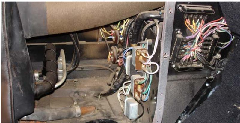
And at left is the maze of wiring and relays to control the rear seat weather. The whole lot could now probably be handled by a small printed circuit!
