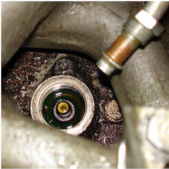
At left we see the evidence of a leaking pump. The pushrod coming up from the camshaft department is also visible. And below is a view of the bottom of the pump showing the base of the pump plunger. It is the gap between these two that broadens with age that gives that characteristic clacking noise common to post55 cars. When replacing the two principal 'O' rings you should also replace the small 'O' ring on the neck of the inlet pie seen at left.
