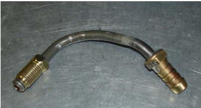
Step one was to make up a new exit pipe from the accumulator. The original was retained in case the scheme did not work
