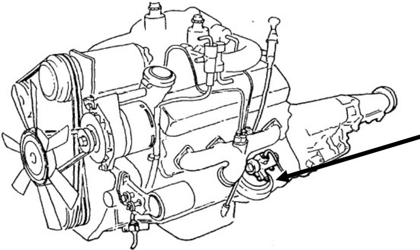
The Shadow 2 engine (chassis numbers 30,000 plus ) had the accumulators repositioned to either side of the engine. This is the number 2 accumulator which for some reason does not generate the knocking noise.
