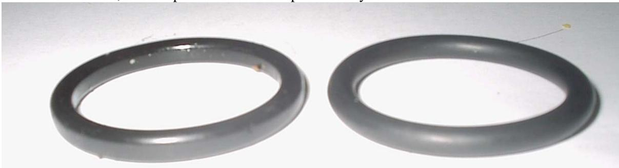
The old 'O' ring removed at left and the new one. Note the flattened outer surface of the old ring where it seals against the outer casing.
