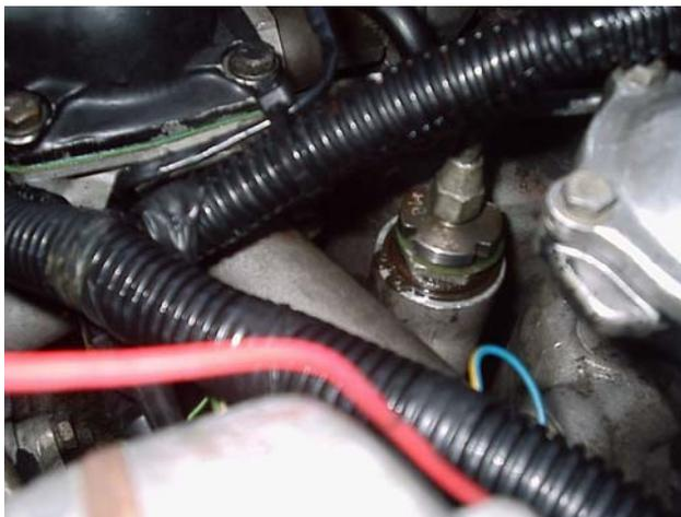
The front pump revealed. Notice the strange 'clover leaf adapter' on the top of the pump which requires a special tool to remove it. The circlip retaining the outer casing can be seen clearly underneath
