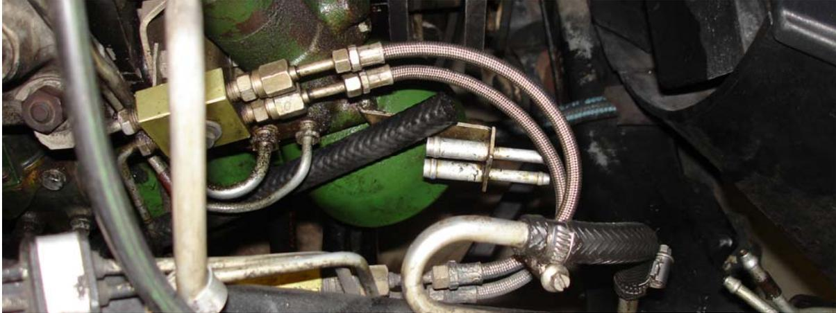
The twin pipe restrictor seen on the Silver Spur in the middle of the picture is mounted on the front of the accumulator valve. The disconnected hose is the large return pipe from the number 2 accumulator located on the side of the engine block. Using this fitting on the T2 obviously used up only one of these restrictor pipes. To the right can be seen the entry ends of the return pipes to the reservoir.
