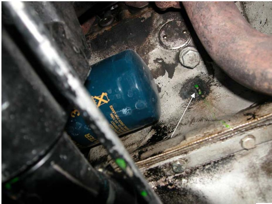
of the cylinder liners on all our vee eight engines have two 'O' rings to seal them in the cylinder block. The bottom one keeps the oil in the sump and the top one keeps the coolant from the sump. The space in between should be empty and dry. Given the vulnerability of 'O' rings generally, the Factory in its wisdom drilled a hole in the block casting midway between the
