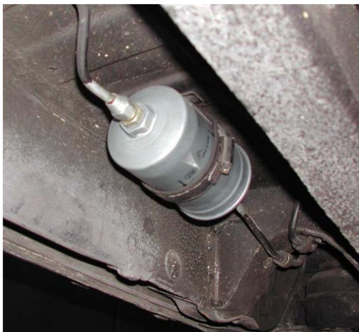
Filters are so easily forgotten. They are easy to change inexpensive and so vital to keeping the car proceeding. Before starting to change one get yourself a clamp to squeeze an upstream flexible line and hold the fuel while you do your job.
