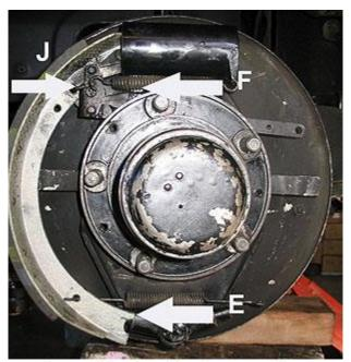
Fig 24. Fitting the trailing shoe assembly at the top end only
