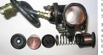
Fig 12. Hydraulic cylinder after having bronze inserts fitted and stainless steel pistons
