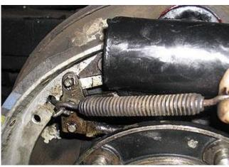
Fig 23 Showing how the retaining spring is fitted onto the "W" link. Use pliers or side cutters to position the spring end into the hydraulic cylinder anchorage
