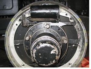
Fig 30. Fitting the locking screw when the intershoe linkage has been set
