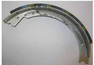
Fig 10. Late type front brake shoe, compare this with the earlier types in Fig 3
