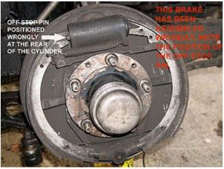
Fig 9. Yet another wrongly positioned off stop pin, even the professionals get it wrong!
