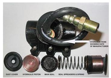
Fig 11. Hydraulic parts of one front brake cylinder, in which cleanliness is essential
