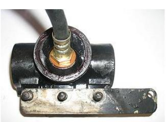
Fig 17. The "W" link anchor plate and cylinder back plate seal, don't forget to position both before refitting the hydraulic cylinder
