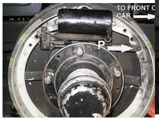
Fig 29. Fitting the link pin
