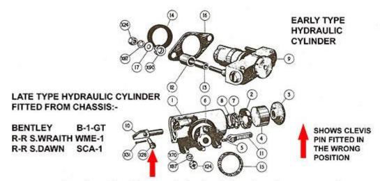
Fig 5. The early and late type hydraulic cylinders, from the parts manual
