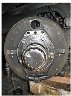
Fig 16. Initial stage of rebuilding, the brake adjuster is fitted loose
