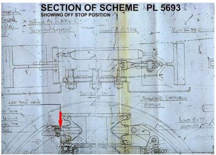
Fig 6. Part of scheme PL 5693, the only printed matter to show the correct layout
