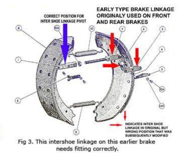
to this day owners are misled by this image. It should be noted that this brake arrangement was also used on the rear brakes right until the "S" series of cars were launched in 1955.
