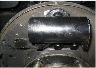
Fig 19. Close up view of the hydraulic cylinder, note the link anchorage hole
