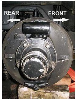
Fig 18. Hydraulic cylinder fitted loosely with the spring anchor plate offset towards the rear
