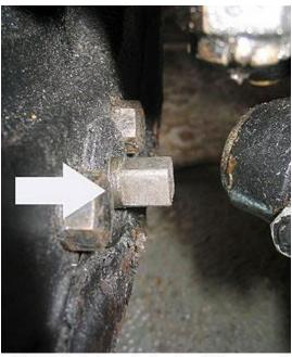
Fig 33. The brake adjuster should be screwed in only a little more than this when the brake has been assembled correctly
