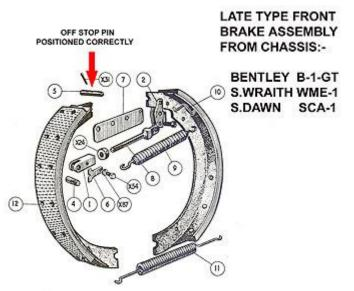
Fig 4. The intershoe linkage of the later front brake
