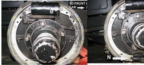
Fig 27. Adding the offstop pin and link
