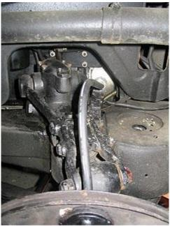
Fig 15. Front brake hose alignment, notice the white dashed line exhibits no twisting
