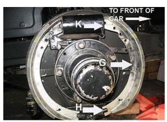
Fig 26. Fitting the leading shoe
