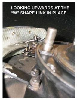
Fig 25 Looking upwards at the "W" shape link in place, owners sometimes find it difficult to latch the link into the anchorage and then fit the return spring
