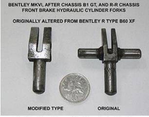
Fig 14. Strengthened front brake fork for the late type front brake
