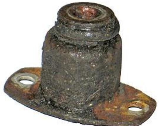
53 year old body mount from under wheel arch showing very poor condition of rubber. Body had dropped on to chassis at rear as is very common
