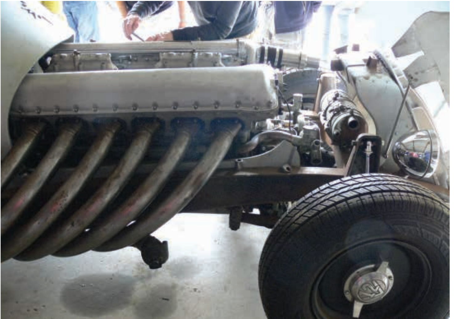
(Clockwise from top) Ivan Shannon's Rolls-Royce Meteor engine sits neatly in his self-constructed chassis; the armadillo-like construction of the tail; a nice period touch of the Pyrene fire extinguisher readily to hand; Ivan explaining a topic in some depth to Ramon Farmer.
