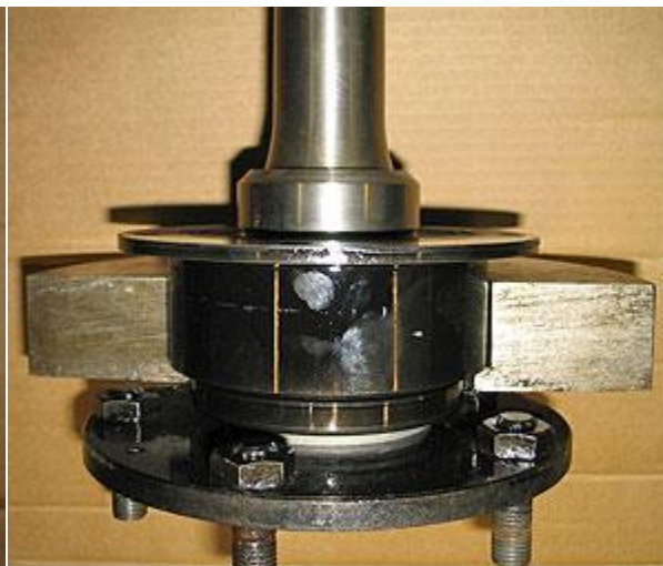
Fig 5. One block shown here, encircling the wheel bearing housing
