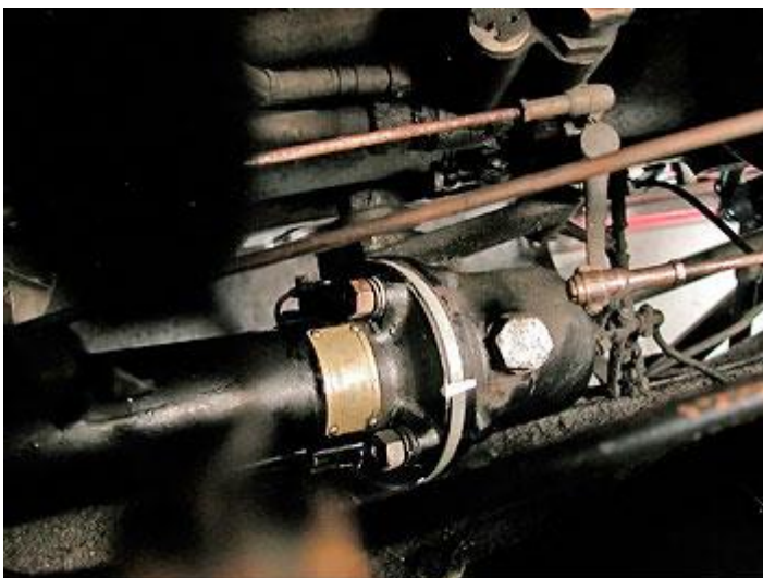
Top view, a white mark on the top of the steering box (the bottom of the box is generally too dirty to put marks on)
