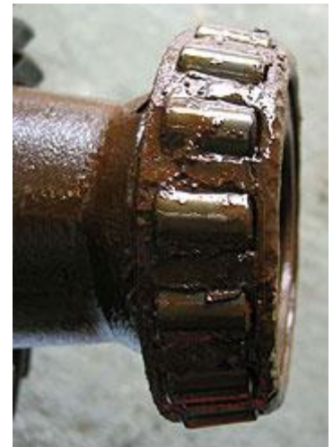
A view of a diff inner axle bearing from the same car. More pertinently, 40 years of sludge developed
