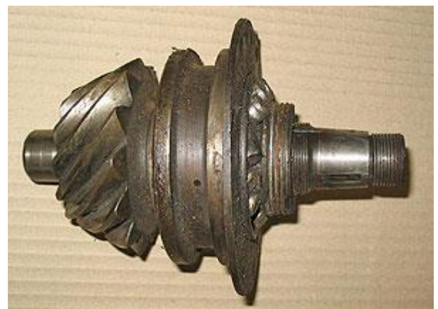
Pinion bearing cage failure and the subsequent lockup
