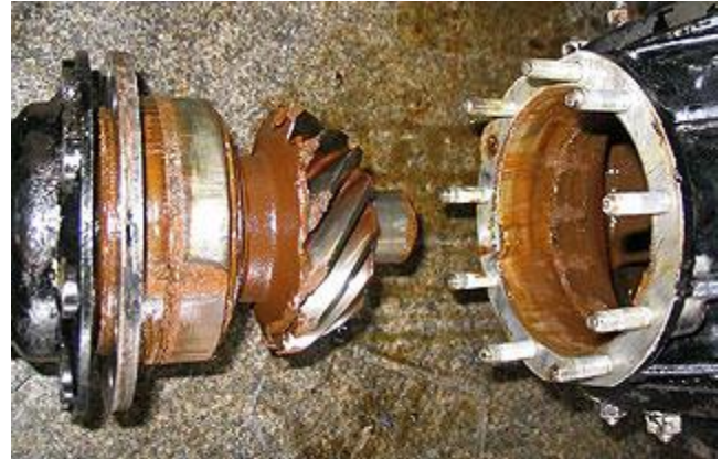
The pinion bearing assembly pulled from the diff casing of an S3 Continental. Note the build up of crud
