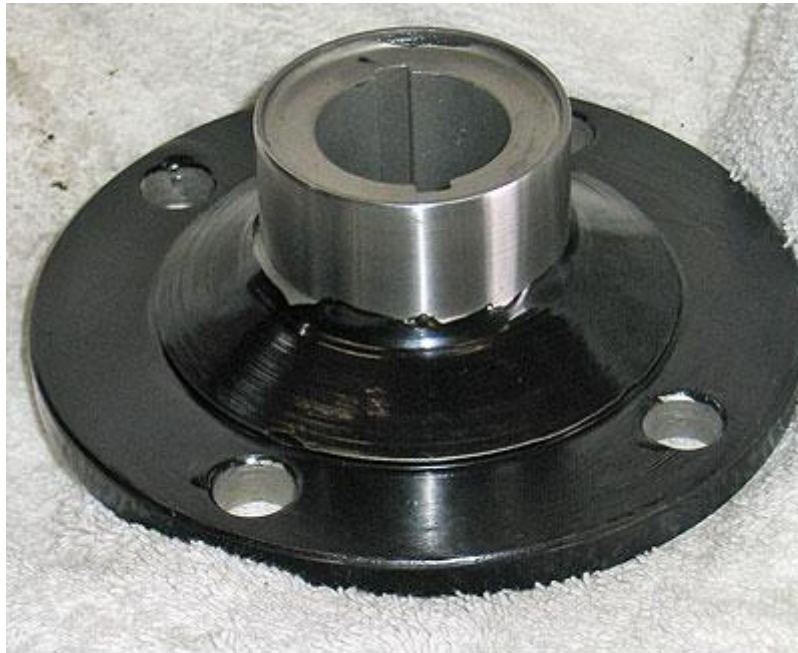
Fig 6. Drive flange machined to accept a new seal, and repainted
