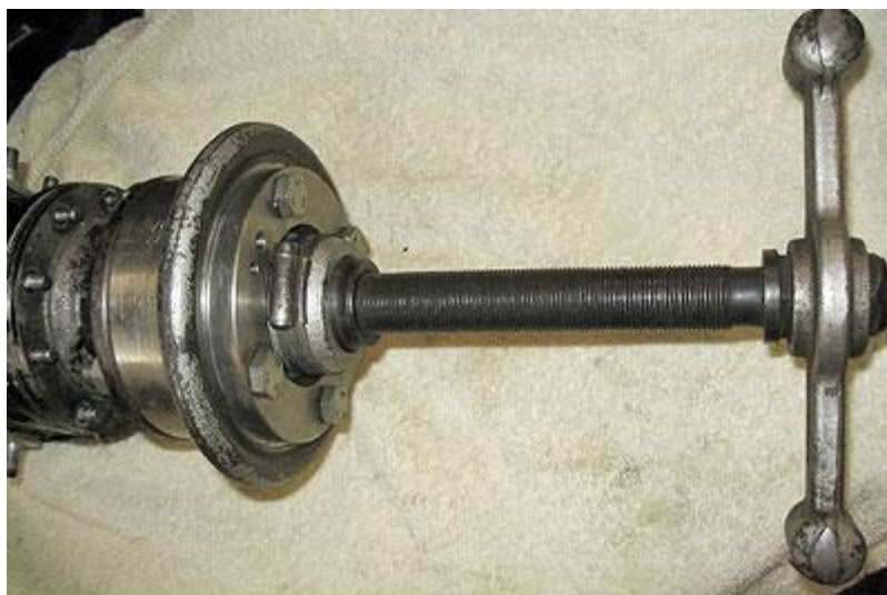
Fig 10. Drive flange puller fitted onto the flange
