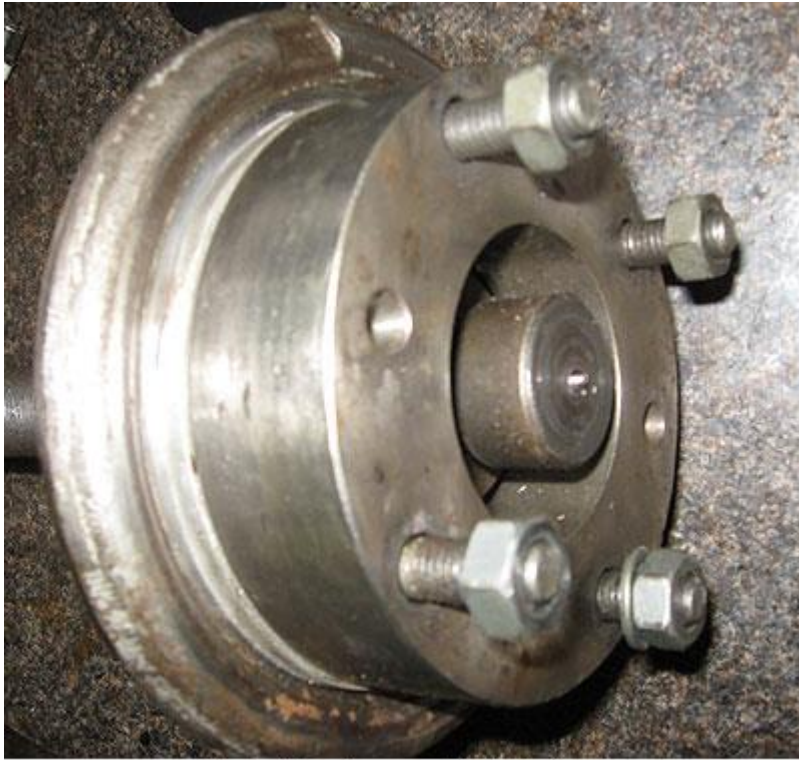
Fig 9. Drive flange puller bolted end
