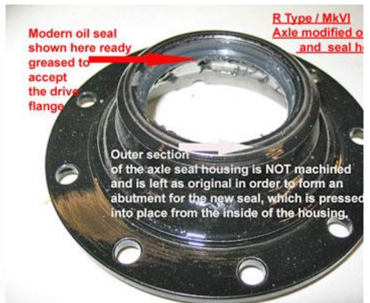
Fig 5. The housing after a modern oil seal has been fitted
