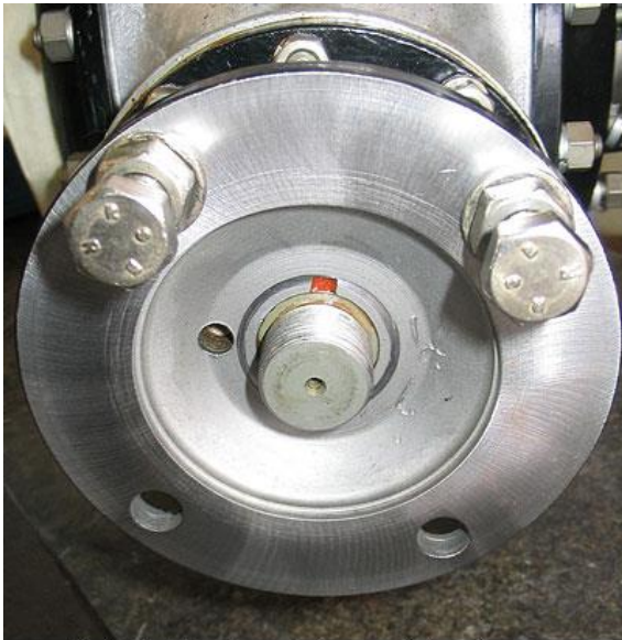
Fig 17. Note how the sealer has spread along the groove after fitting the flange
