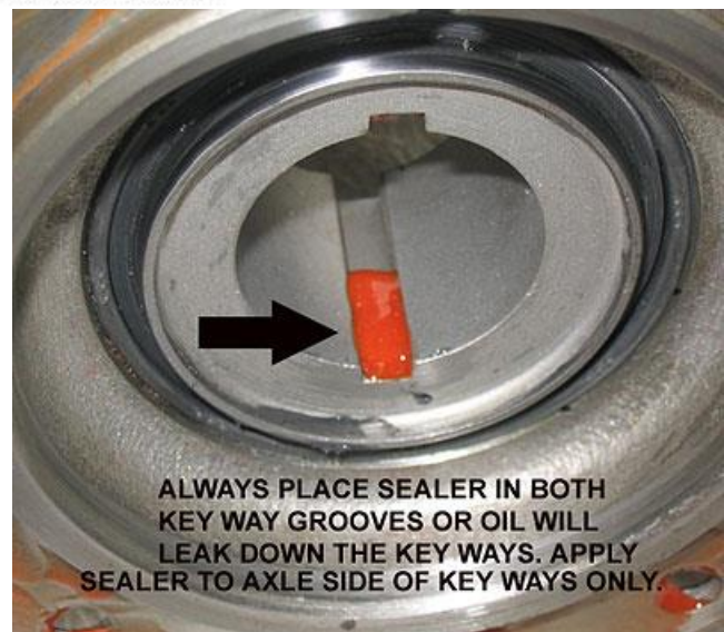
Fig 16. Sealer placed in the key way groove from the inside of the flange
