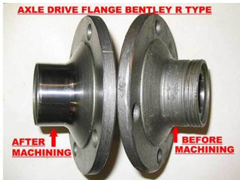
Fig 2. Comparison of old and remachined seal running surfaces on an axle flange
