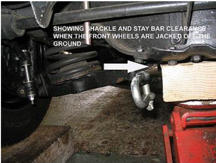
Fig 5. The new bar clears the front cross member on suspension rebound with shackle positions some 3 inch forward of the existing front setscrew attachment point
