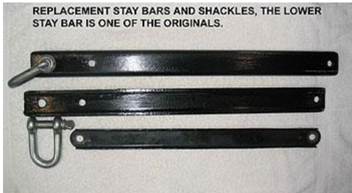
Fig 2. Comparison of the parts, new and old, shown here with shackle holes 3 inch forward
