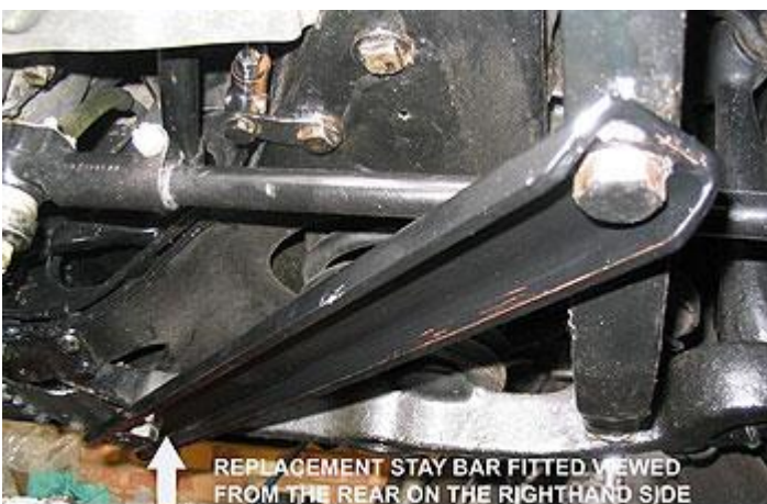
Fig 7. New bar fitted, note the increased thickness compared with Fig 1
