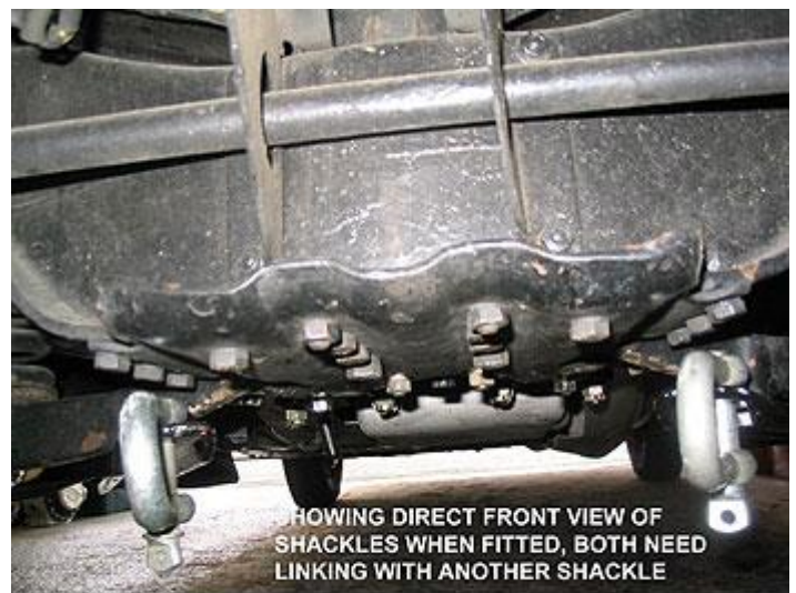
Fig 10. For towing integrity the shackles need loosely joining with a rope or another shackle
