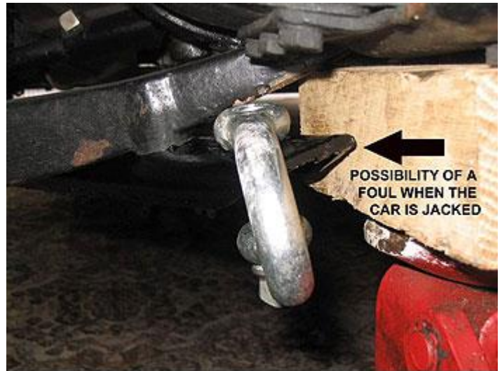
Fig 6. Clear of the chassis fixtures but a possible foul with your favourite jacking block
