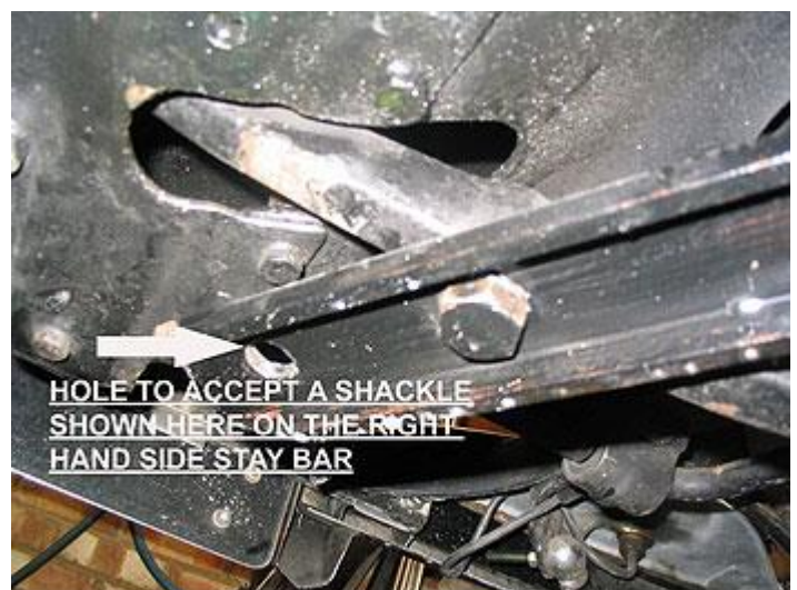
Fig 8. The extra sway bar hole, ready to accept one of the two shackles in an emergency
