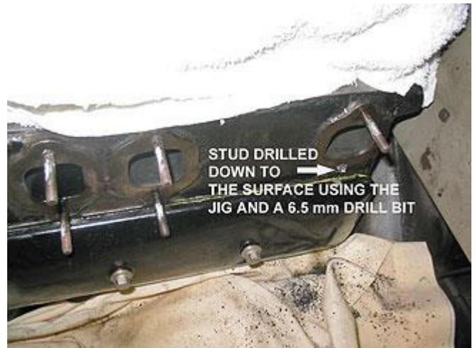
Fig 5. Stud drilled down to the block face
