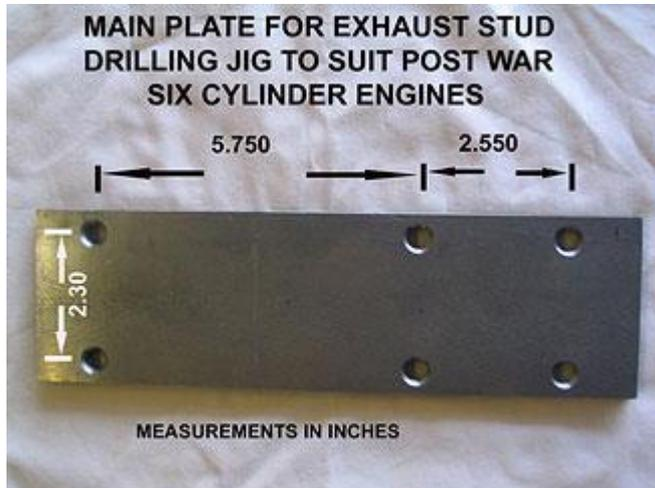
Fig 2. Jig plate dimensions
