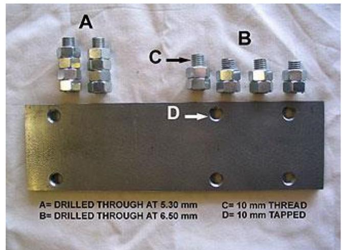
Fig 3. Jig plate with guides of two bore sizes
