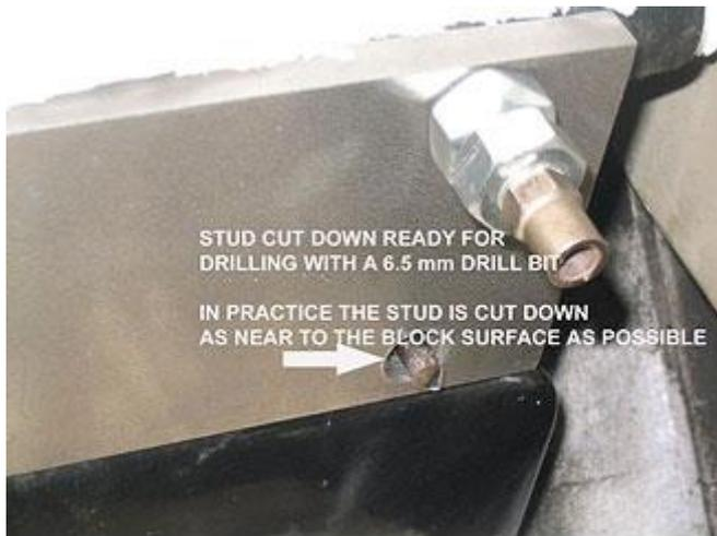
Fig 4. Stud cut off and jig plate fitted, now waiting a 'B' type guide screwing in over the stud
