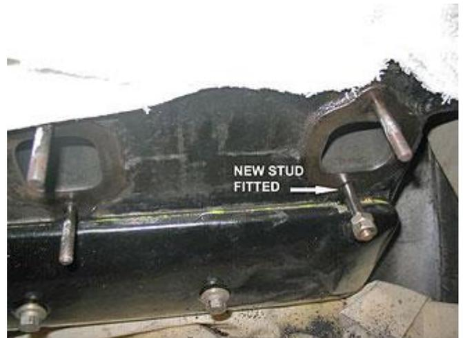
Fig 9. Stud successfully fitted, accurately and without damage
