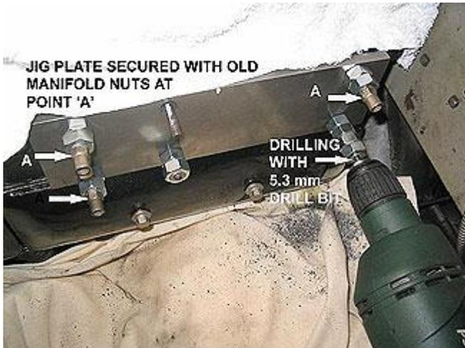
Fig 7. Pilot drilling with 5.3 mm drill ready for taper tapping
