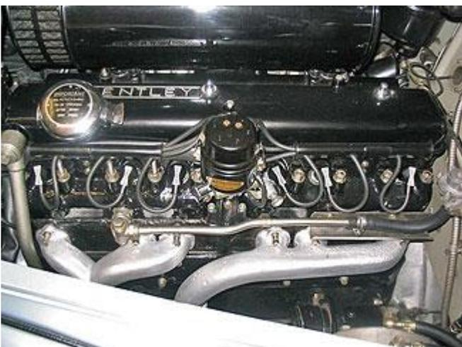
Fig 10. Manifolds replaced
