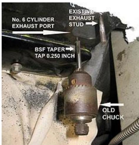
Fig 8. Using an old drill chuck to tap in a restricted space
