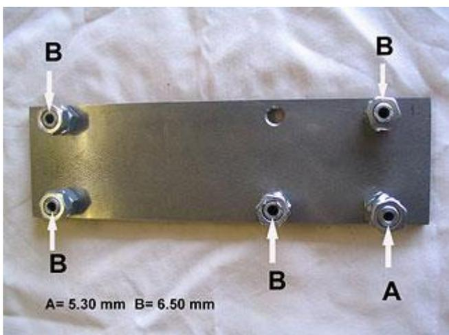
Fig 6. Jig configuration before final drilling of the lower rear manifold stud
