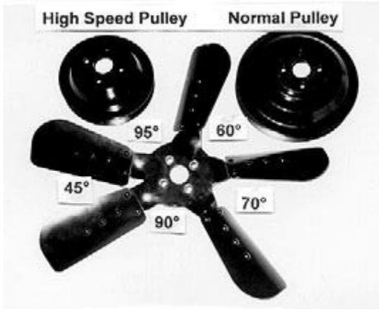
FIG9. High speed pulley, normal pulley and RE 6060 Fan assembly.
