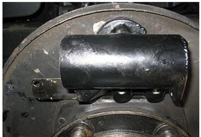
Fig 19. Close up view of the hydraulic cylinder, note the link anchorage hole
