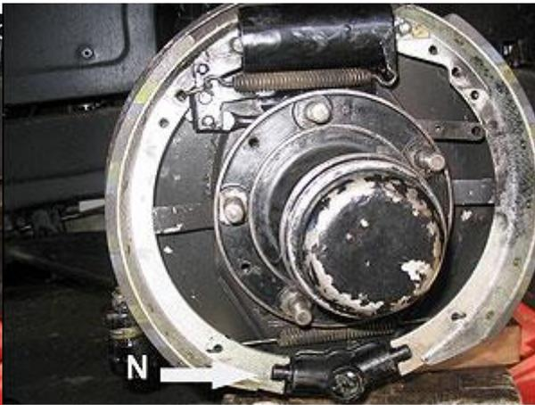
Fig 28. Fitting the trailing shoe at the brake adjuster end
