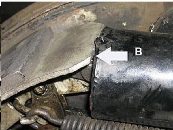
Fig 32. There will be gap between the trailing shoe and the wheel cylinder, and it could be larger than the gap that is shown
