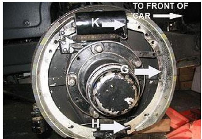
Fig 26. Fitting the leading shoe
