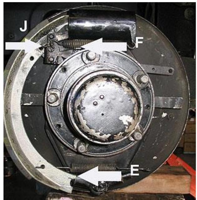
Fig 24. Fitting the trailing shoe assembly at the top end only
