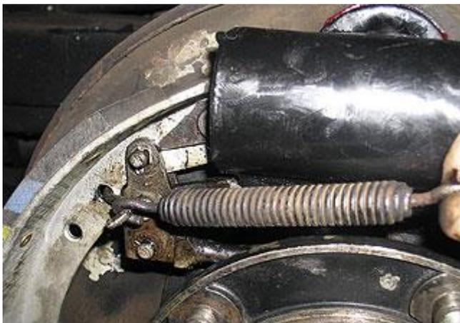
Fig 23 Showing how the retaining spring is fitted onto the "W" link. Use pliers or side cutters to position the spring end into the hydraulic cylinder anchorage
