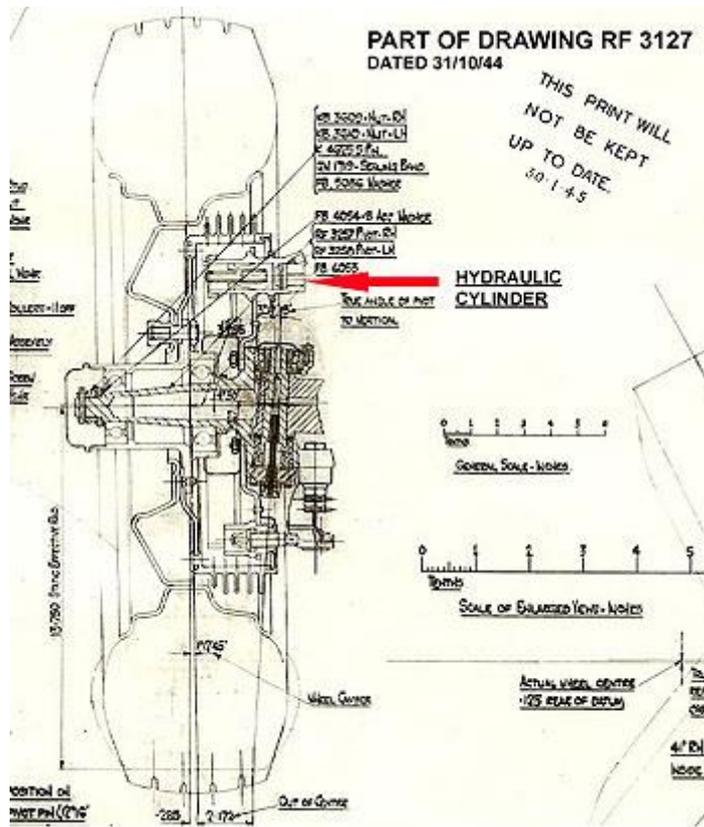
Fig 2. Part of the October 1944 drawing RF 3127 showing a hydraulic cylinder.
