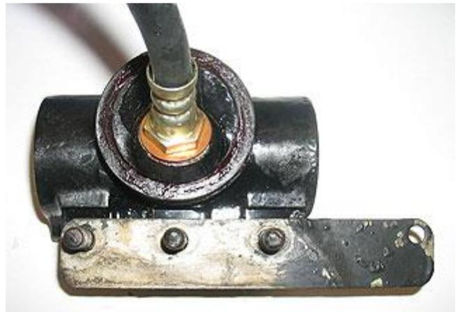
Fig 17. The "W" link anchor plate and cylinder back plate seal, don't forget to position both before refitting the hydraulic cylinder
