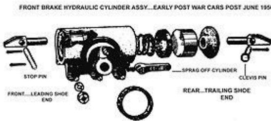
Fig 7. The corrected late type hydraulic cylinder assembly
