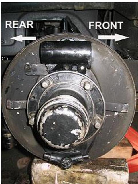
Fig 18. Hydraulic cylinder fitted loosely with the spring anchor plate offset towards the rear
