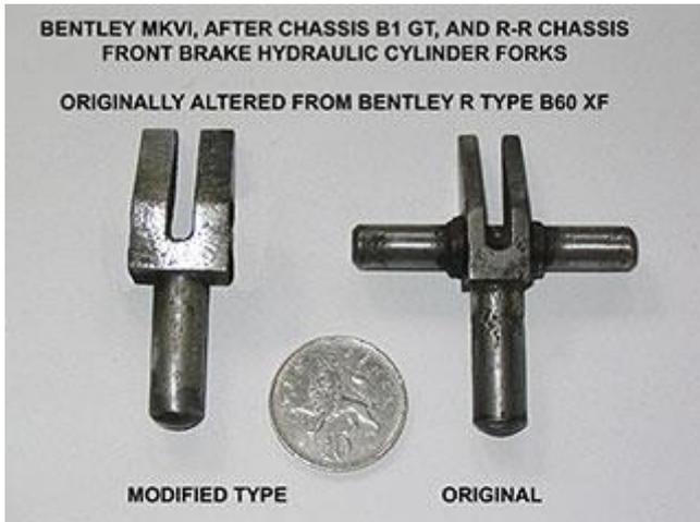
Fig 14. Strengthened front brake fork for the late type front brake
