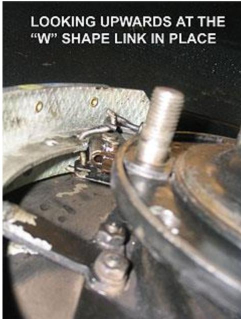
Fig 25 Looking upwards at the "W" shape link in place, owners sometimes find it difficult to latch the link into the anchorage and then fit the return spring
