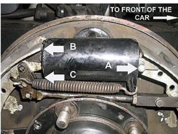
Fig 31. Points to check when the brake has been assembled
