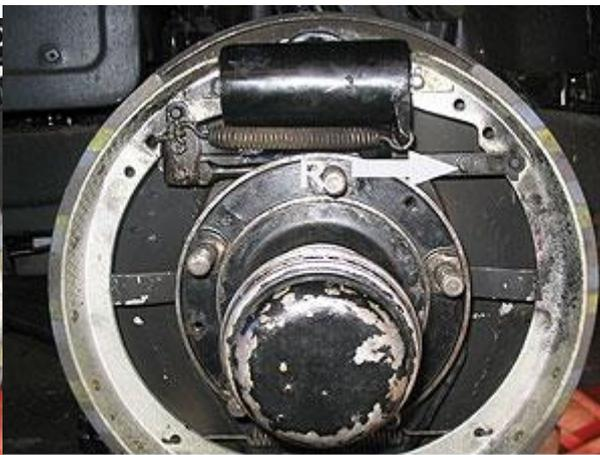
Fig 30. Fitting the locking screw when the intershoe linkage has been set
