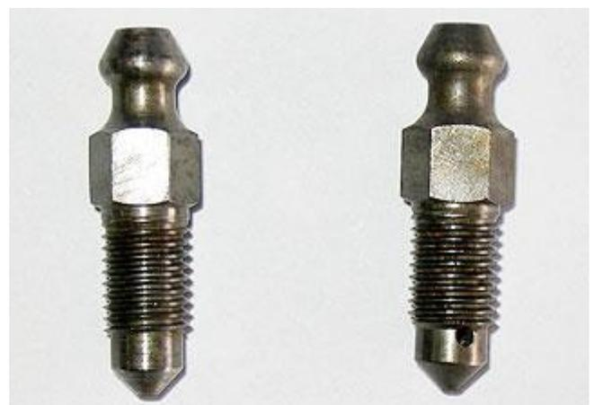
Fig 13. Late type front brake bleeder with Whitworth form thread, these are none standard!
