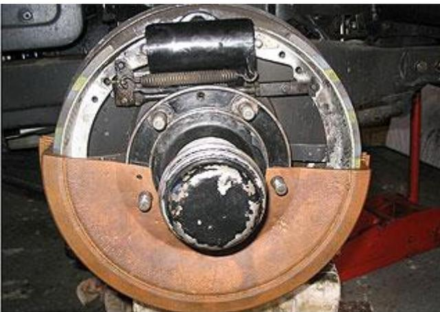
Fig 22. Viewing the results using a test drum if you are lucky enough to possess one!
