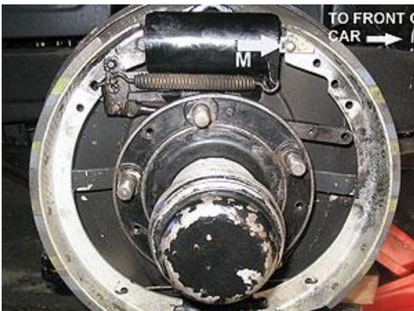
Fig 27. Adding the offstop pin and link
