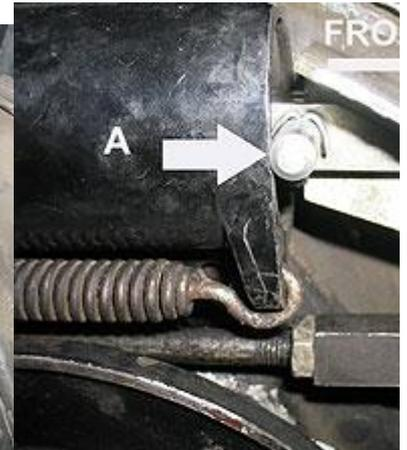
Fig 21 Showing the objective, fit far forward as possible with against the cylinder
