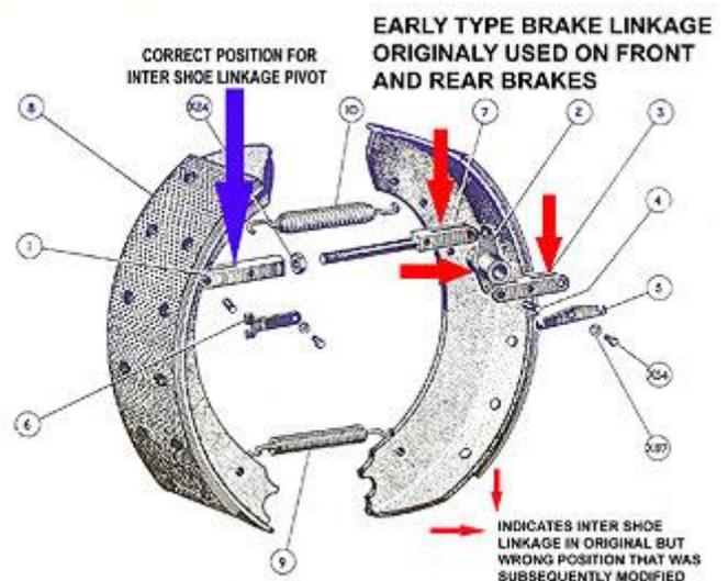
Fig 3. This intershoe linkage on this earlier brake needs fitting correctly.
