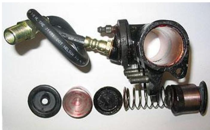
Fig 12. Hydraulic cylinder after having bronze inserts fitted and stainless steel pistons
