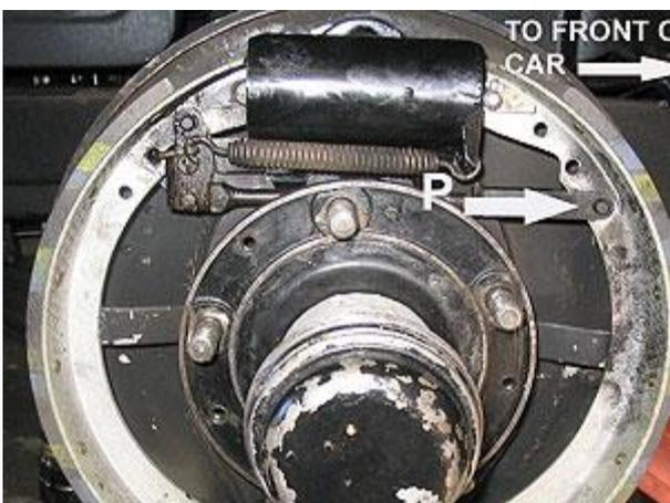
Fig 29. Fitting the link pin
